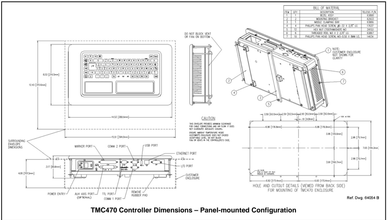
**TMC470 Controller Dimensions – Panel-mounted Configuration**
