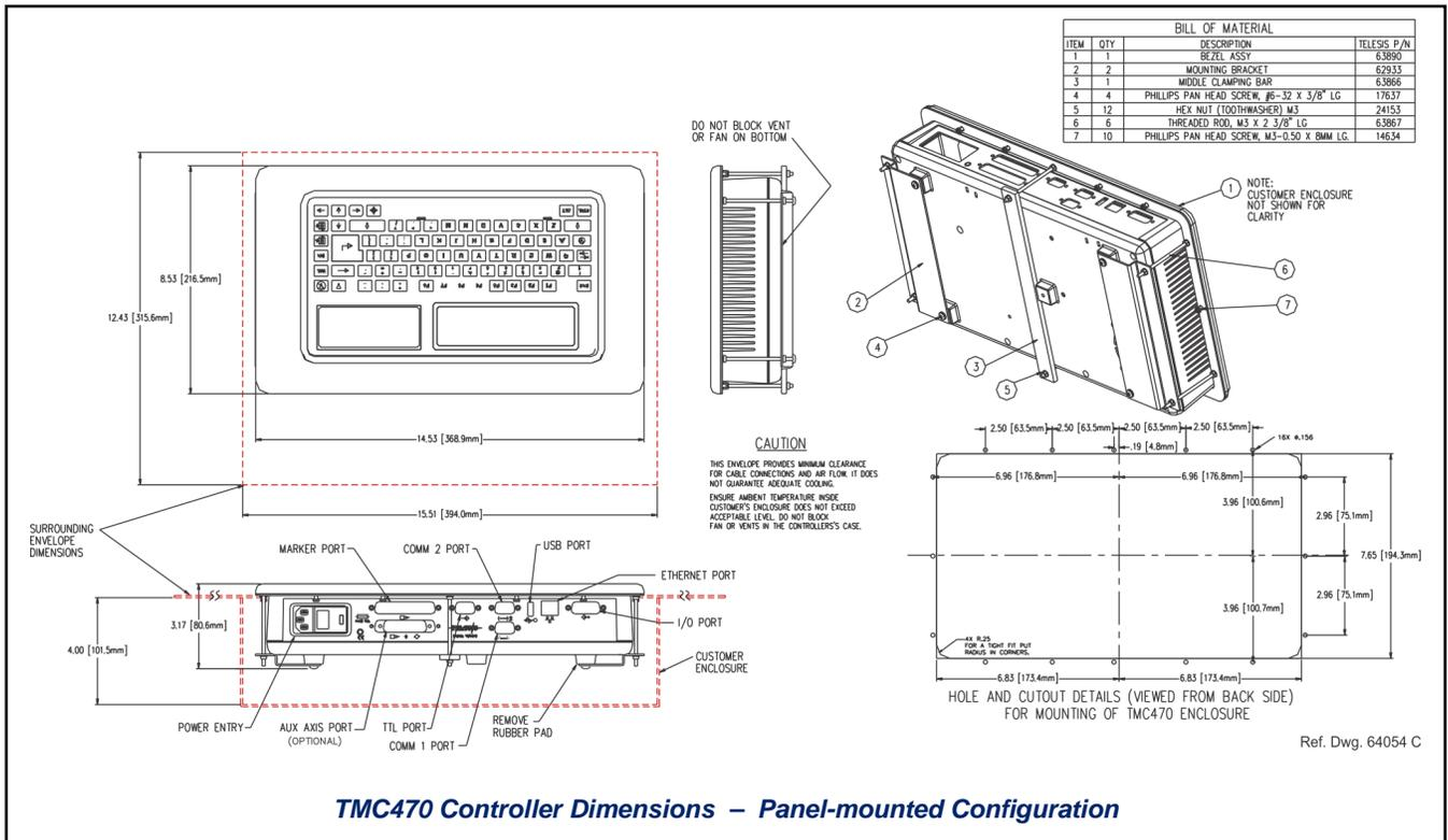
**TMC470 Controller Dimensions – Panel-mounted Configuration**
