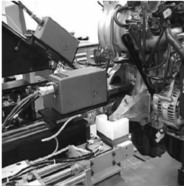
The transmission marker approaches the assembly at a 35° angle and the engine marker is mounted horizontally. Both markers and the clamp (bottom) approach the assembly on pneumatic slides.
