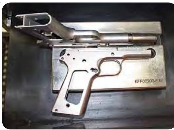
Ruger has developed several fixtures that hold parts exactly in focus for custom laser-etching machines, which are now used to cut nearly all the markings on Ruger firearms parts, including serial numbers.
